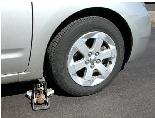
Lift location, before using the jack.
