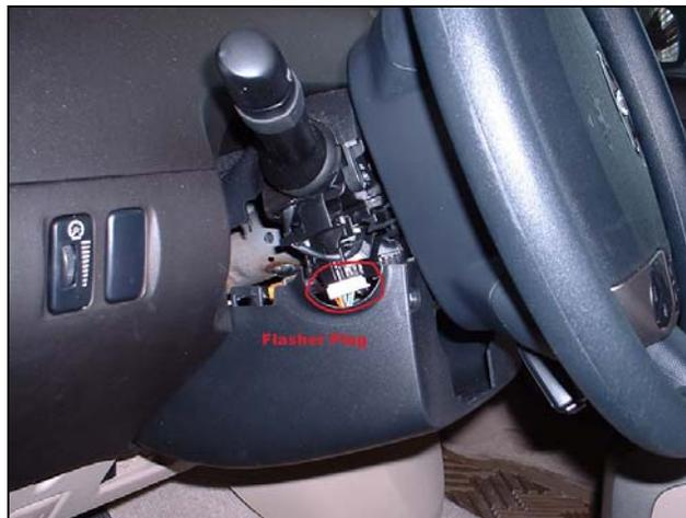
2) Locate and unplug the white flasher plug visible just on the left side of the bottom of the steering column.
