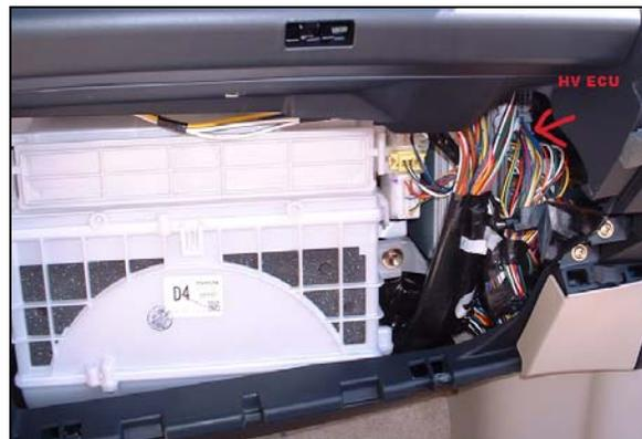
There are 3 vertically oriented ECUs, 2 with white. The HV ECU is the one farthest to the right and is the only one with gray plugs.
