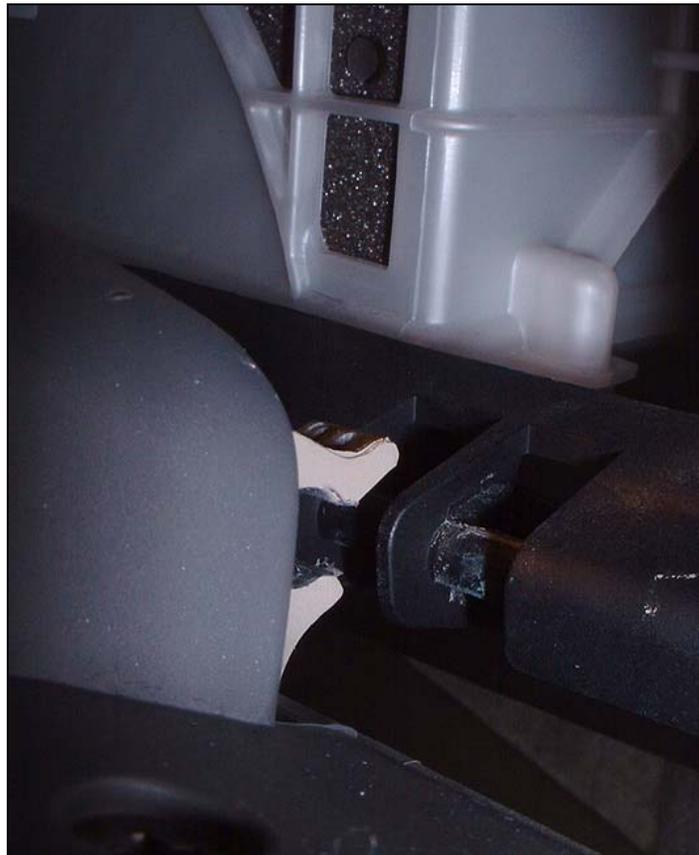
You may also need to unclip the little hydraulic piston that keeps the door from falling open too quickly. Next, grasp the bottom of the silver vent piece next to the glove box. Pull it toward you firmly. It should unclip at the bottom first. Then pull the whole unit straight out.
