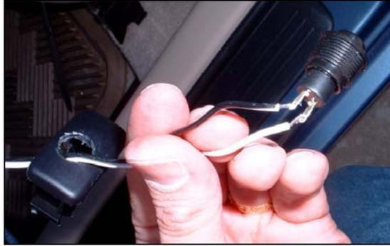
You may not be able to get the nut flush due to the residual fins, but it doesn't matter as long as the button is secure. Now solder the wires to the connectors on the button. **DON'T** overheat the connectors, as it could damage the button's internal contacts. (It doesn't matter which wire goes onto which contact.)
