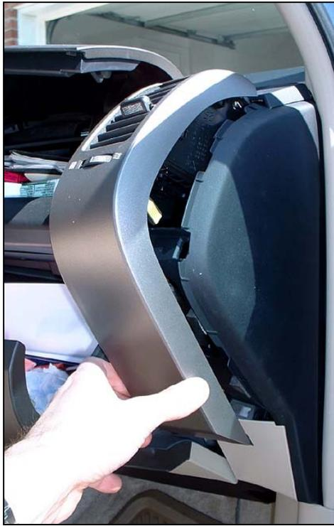
You'll eventually need to remove the driver's side (far left) vent piece as well. Finally, remove the smaller square plastic piece just below the passenger side vent--it pulls straight out.
