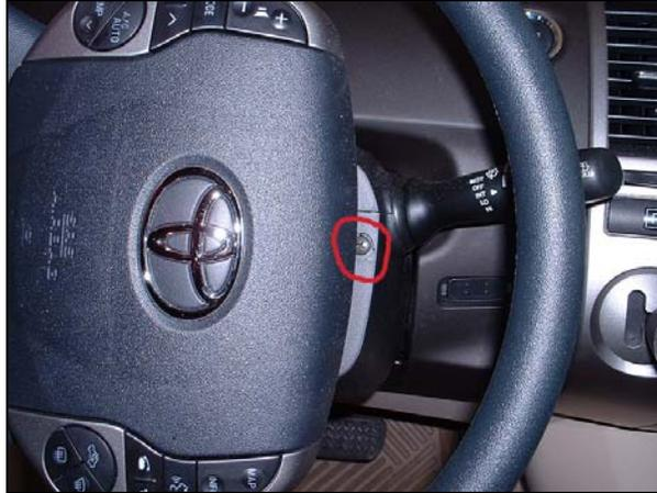
Then turn the wheel 180 degrees left (90 degrees from normal position) and remove the black screw on the left side of the steering column.
