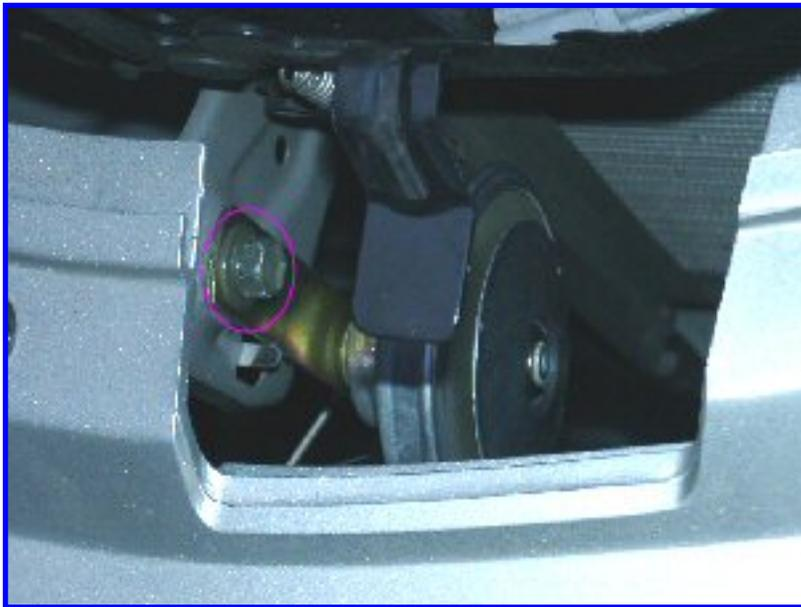
If your aftermarket horn is like most, it can be set up for either 1 or 2-wire installations. If so, simply use the ground wire that should have been included with it, remove the horn from its mounting bracket if already bolted to it, and bolt the harness between the horn and mounting bracket. Then plug the wire into one of the horn terminals (check the install directions to see if it matters which terminal to plug it into - on most horns it doesn't matter, but it might on some).
