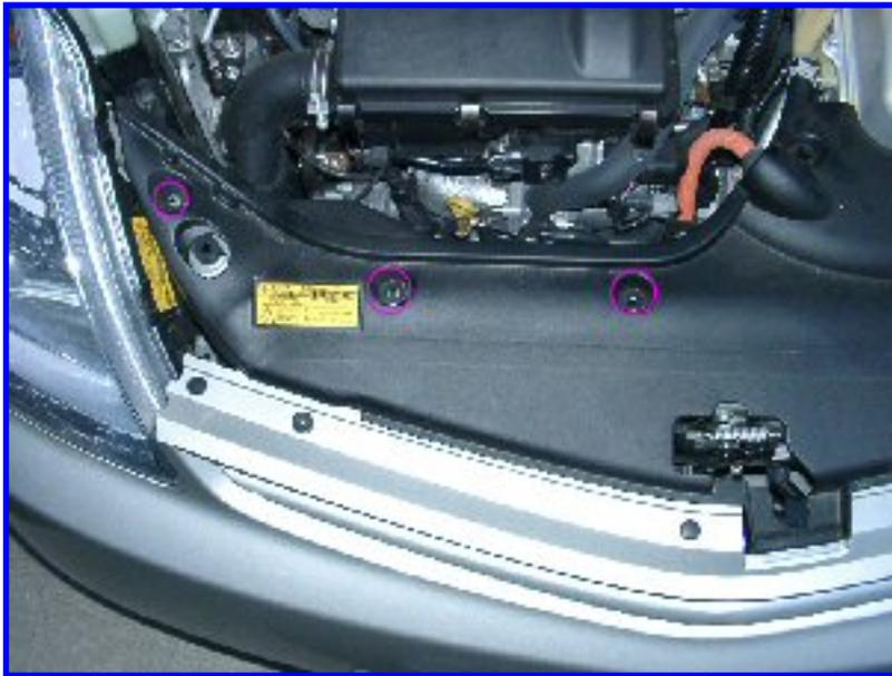
until you see the center of the pin lift up a little, then hook a fingernail or small flatblade screwdriver under the pin center, remove the Philips screwdriver, and lift up on the pin.
