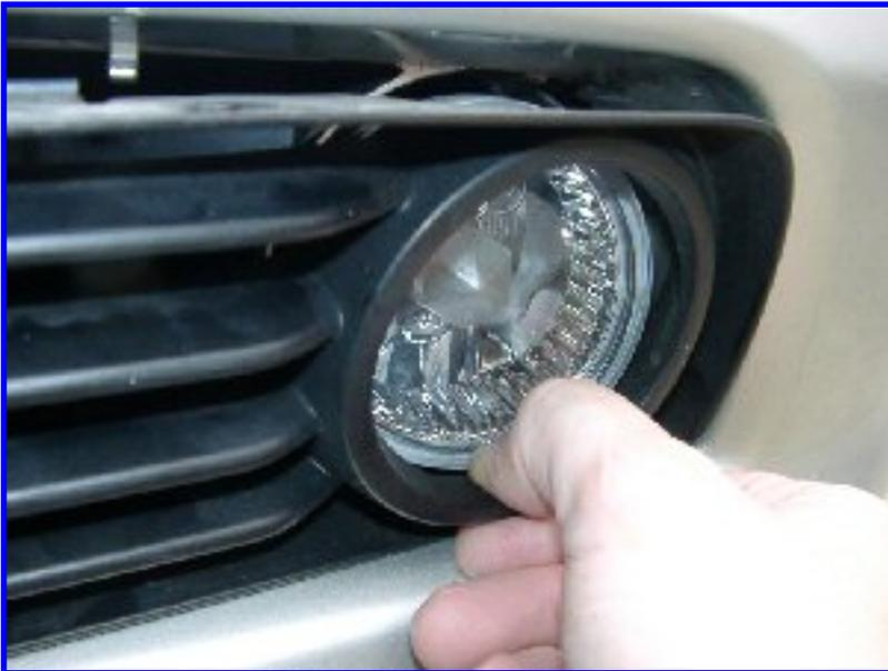
The bottom right tab is a bit tougher, to avoid breaking the grille, grab it here and wiggle it around.
