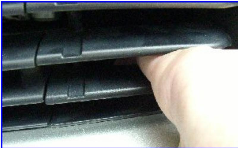
I stuck my finger through the second from bottom slot to lift up on the tab. If you have smaller hands, you might be able to pull it from the bottom slot. Lift the tab up, and pull the foglight grille forward.
