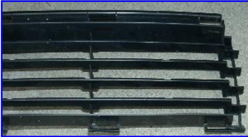
Here you can see the bottom tabs on the grille, at the bottom of the picture. This is why the grille has to be pushed *into* the nose, not pulled out of it.
