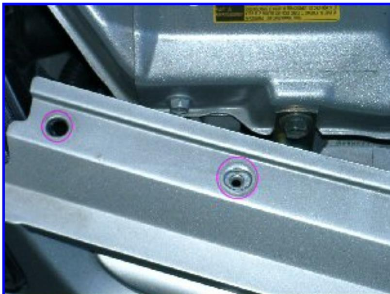
You only need to remove 2 fasteners in front of the horn to make it very easy to access it. The circle on the left is for a push-pin style, simply lever the center of the pin up with a flatblade screwdriver, and pull the pin out. The circle on the right is for a hood bumper, just use a Philips screwdriver to remove it.
