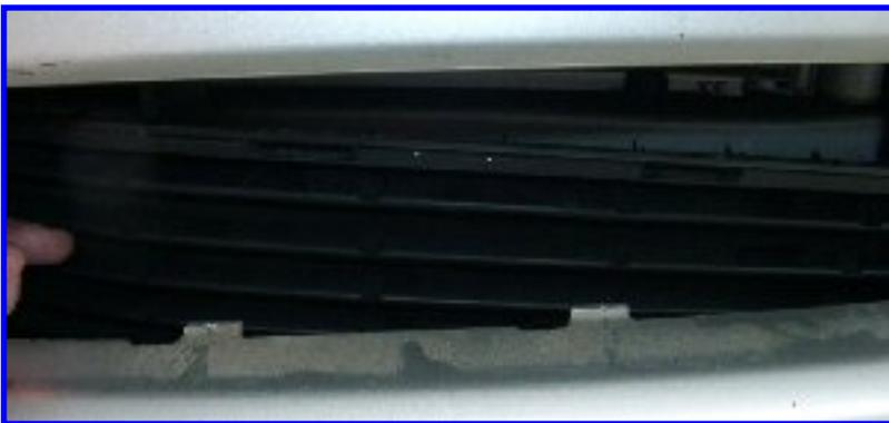
Once all the tabs are free, push the grille into the opening. You might have to move it around a bit to get it past the edge of the nose opening.
