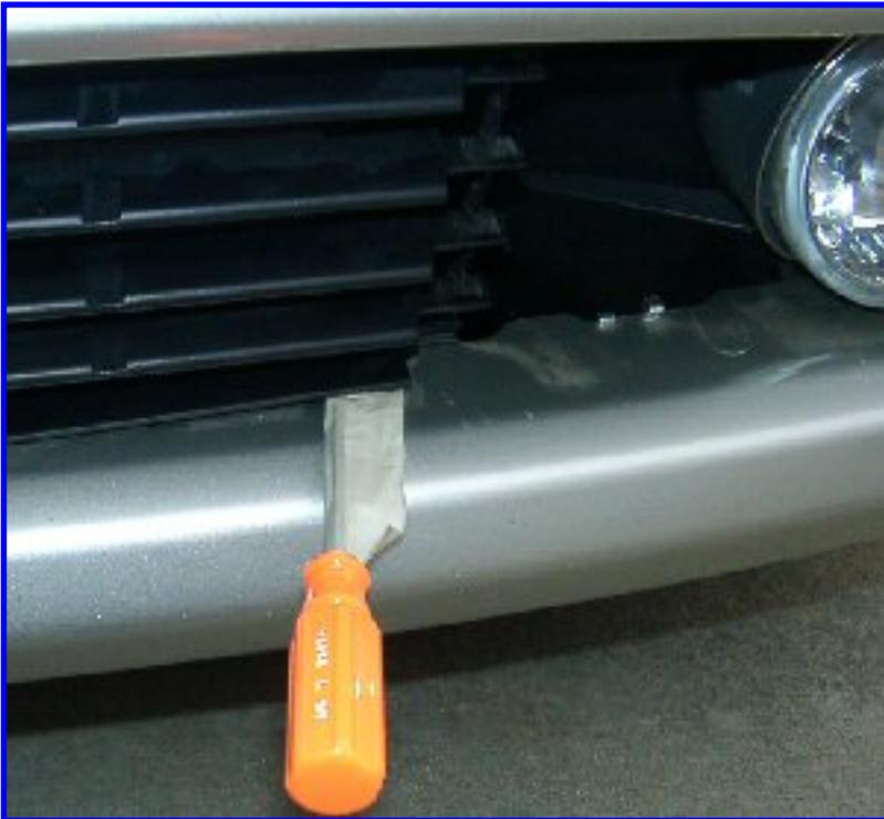
The bottom tabs are tough to locate. Even in daylight, you may need a flashlight to properly highlight them. Again, insert the screwdriver between the nose and grille, wiggle it around, and push the grille towards the radiator until the tab pops free.
