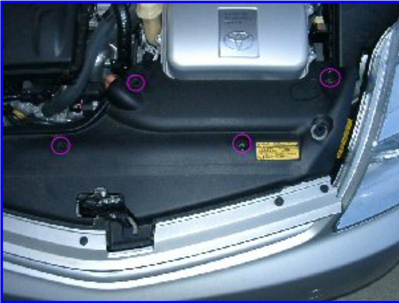
Start by removing the fastening pins circled here...
