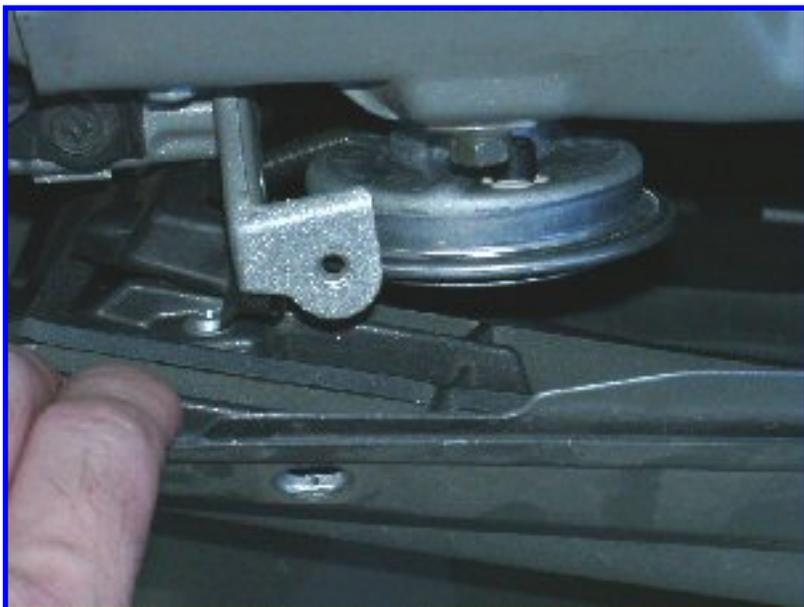
Once the 2 fasteners are out, simply grab the grille and pull forward as much as needed to access the horn. I personally would not yank the heck out of it, but as you can see, you can flex it quite a bit without hurting anything (the paint on the bumper has a flex additive).
