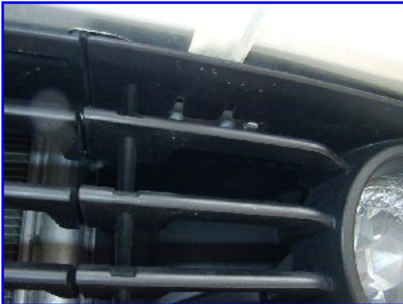
You can try a finger with the upper left tab, but it didn't work for me, so I covered a screwdriver with tape as noted in the Shop Manual. NOTE - it is best to use at least 2 layers of tape. Press the small screwdriver between the tab and bumper, and wiggle it around until you can pull the grille forward.
