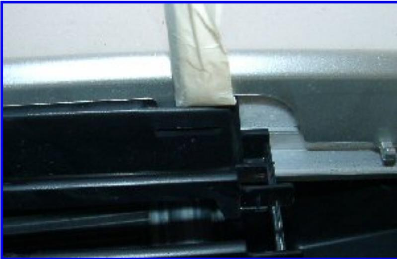
Wedge the screwdriver between the nose and grille, wiggle it around, and push the grille inwards towards the radiator.
